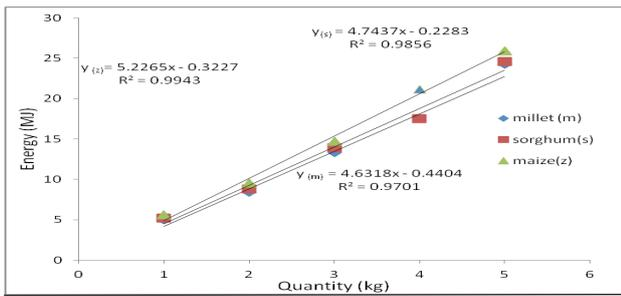
Figure 1. Energy input in dry milling of selected grains
