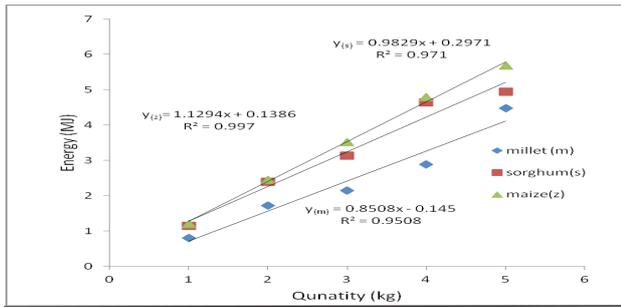
Figure 2. Energy input in wet milling selected grains
