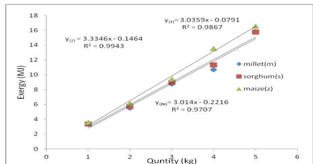
Figure 3. Exergy pattern in dry milling selected grains
